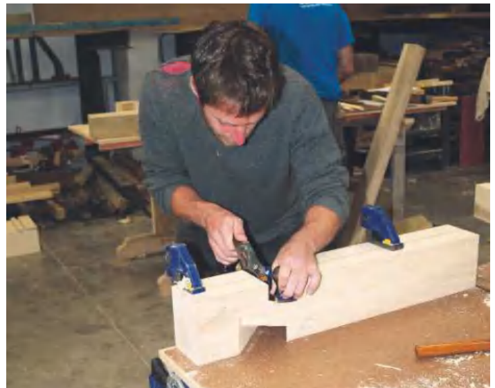
▲ Pic.10 Lap joint floors were cleaned up with rebate planes. The American tulipwood was fairly kind to work
